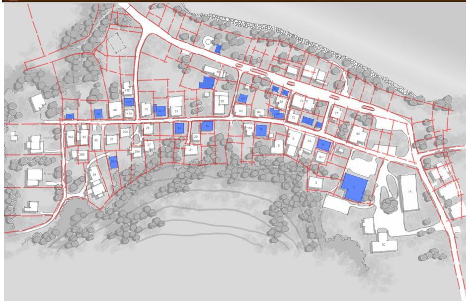
Structures highlighted in blue are in poor condition and pose life-safey threats in the District. Interpolated District property lines are shown in red dashed lines.
